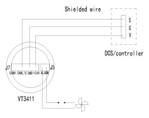
The wiring of detector can be seen in Fig. Pay attention to the following contents when wiring:
