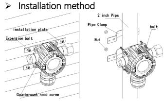
As shown in Fig, the detector can be installed by tube clamp or wall-mounted method according to site operating conditions. For tube clamp mode, the general 0.75~2inch steel tube; for wall-mounted mode, the wall surface shall have enough strengthen to support and firmly fix the detector.
