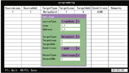
Click the "OK"key,input password and enter the Autocontrol interface→Click the "F2"key pop-up dialogue box→Manually added according to field components. In the linkage programming, the linkage source is the on-site detection device, and the linkage purpose is the output device (including the sound and light alarm, the linkage module, etc.), and the linkage logic is to use the linkage source to linkage linkage purpose, and each linkage source needs to separately add linkage.
